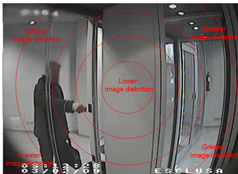
Figure B14 Example of lens barrelling distortion in an image
