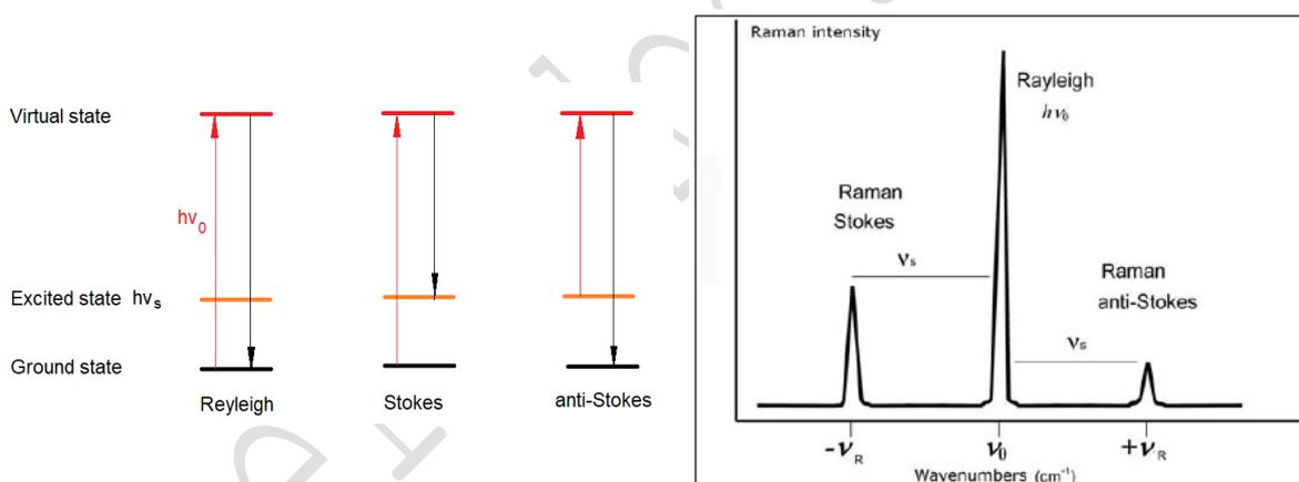
Stokes and anti-Stokes peaks are symmetrically positioned about the Rayleigh peak but the former is more intense. As the effects are weak and fluorescence can overwhelm the peaks, Raman spectra are usually recorded in the Stokes region only. Monochromatic excitation is performed using laser sources.
