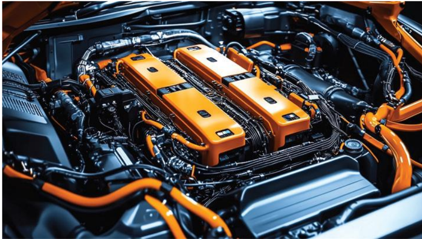
Figure 15. Highlighted parts that may pose an electrical hazard under an EV's bonnet
